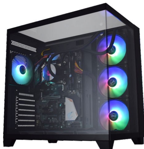
WATER COOLER INSTALADO NO GABINETE
