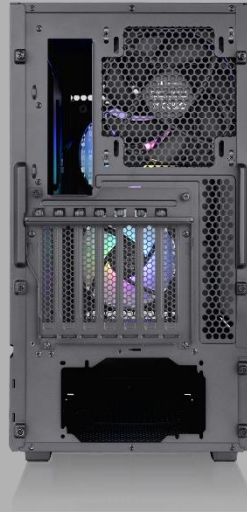
Vertical VGA installation
