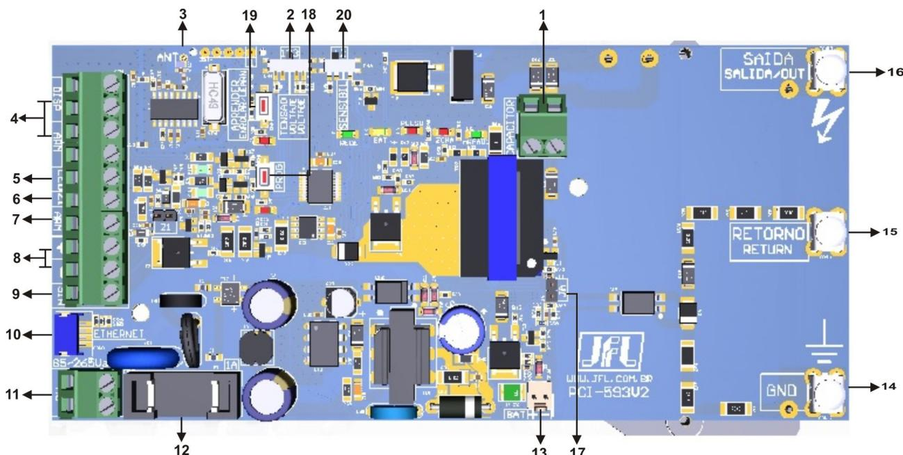
1. Conector do capacitor 5  $\mu$ F/440 Va.c. (ECR-18 Plus) e 40  $\mu$ F/250 Va.c. (ECR-18i Plus).
